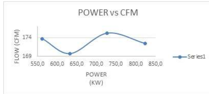
Figure 5. Example of measuring flow vs. rated power of a compressor. Source: Research Team.
